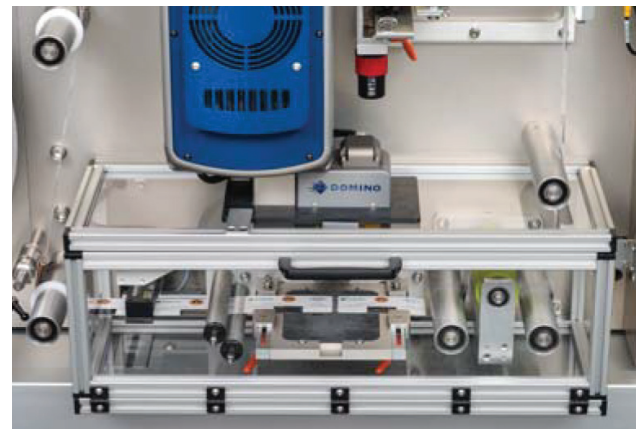
SHOWN WITH LASER PRINTER AND CODE PRESENCE VERIFICATION CAMERA OPTIONS
